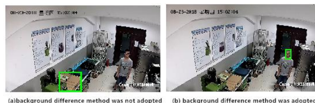
Fig. 5 Influence of background difference method on face detection: (a) background difference method was not adopted (b) background difference method was adopted
