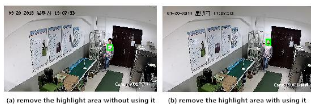
Fig. 6 The influence of whether to use highlight region removal on the correct detection of face: (a) remove the highlight area without using it (b) remove the highlight area with using it
