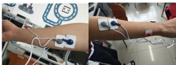
Fig.2 sEMG signal acquisition module - electrode placement
