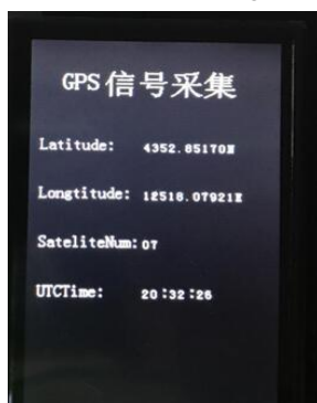
Fig. 5 The results of GPS signal acquisition (display latitude, accuracy, number of analytic satellites, time by row)
