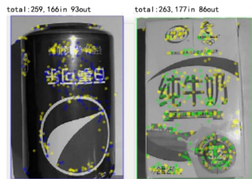
Fig.5. SIFT algorithm image matching results
