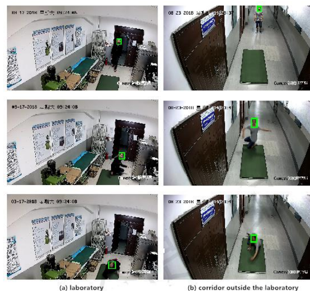
Fig. 7 Correct face tracking under different scenes : (a) laboratory, (b) corridor outside the laboratory
