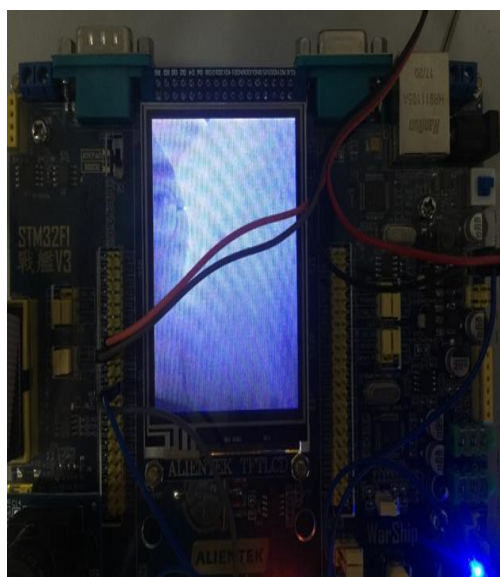
Fig.10 OV7670 camera captures images in real time
