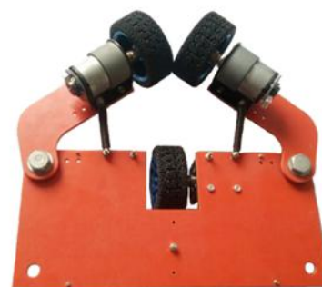
Fig.3 Structure Physical Chart of Rod-climbing Robot
