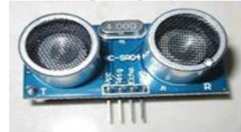
Fig .2. HC-SR04_Module physical map
