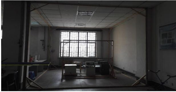
Fig.9 Traiaxial square coils device
