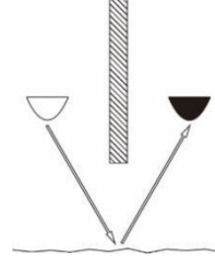
Fig.4 The grayscale sensor is used to detect the principle of the filter
